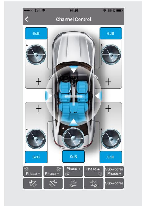
In the lower area of the menu in the top line are the icons for setting the phase. From left to right: Front left, Front right, Rear left, Rear right, Subwoofer.
